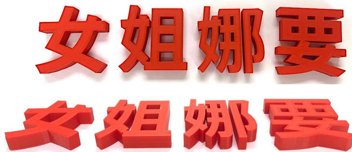
Figure 1 Pictures of 3D Printed Characters: 女、姐、娜、要
